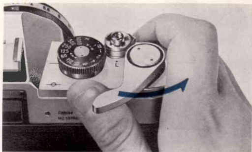
4. Wind the film advance lever.
