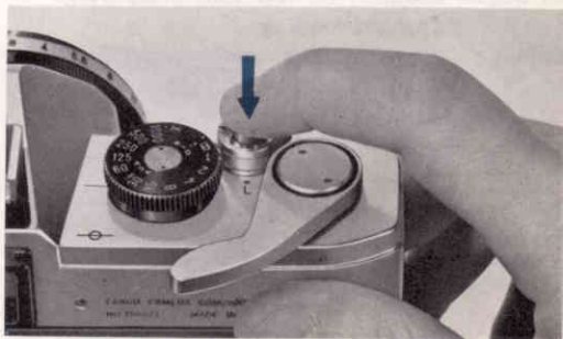
8. Press the shutter release button.
